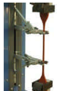
Extensometer arms closed and engaged with sample
